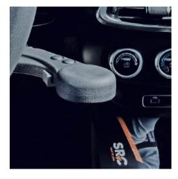
CONTROL UNIT INFRARED CONTROLS PEDAL ON THE LEFT
